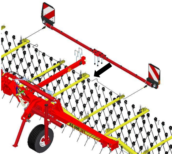
Figure 11: AS 600 M1 – installing the lighting
