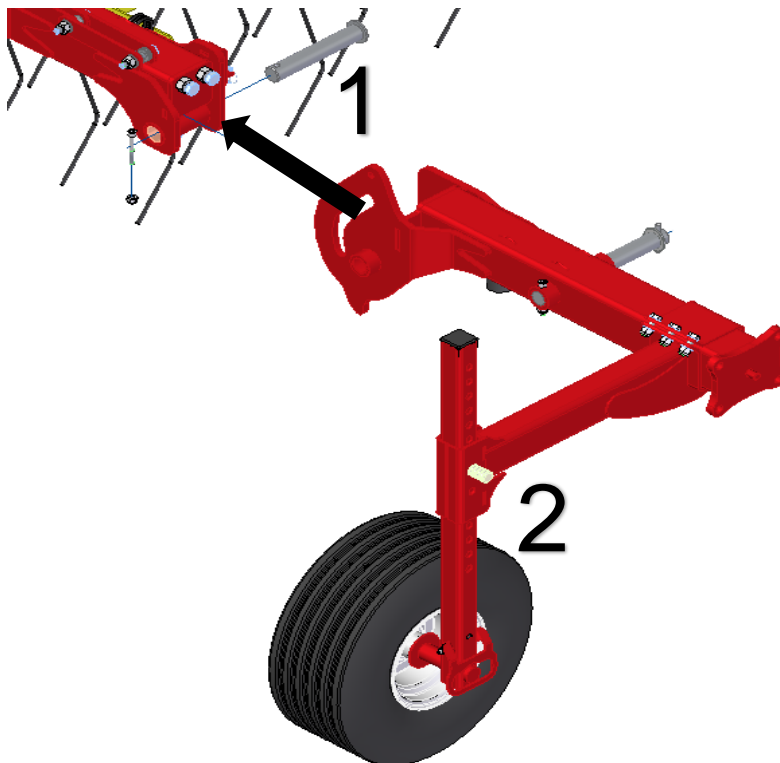
Figure 20: Installing the side frame on the main frame of the AS 900 M1 scissors folding unit
