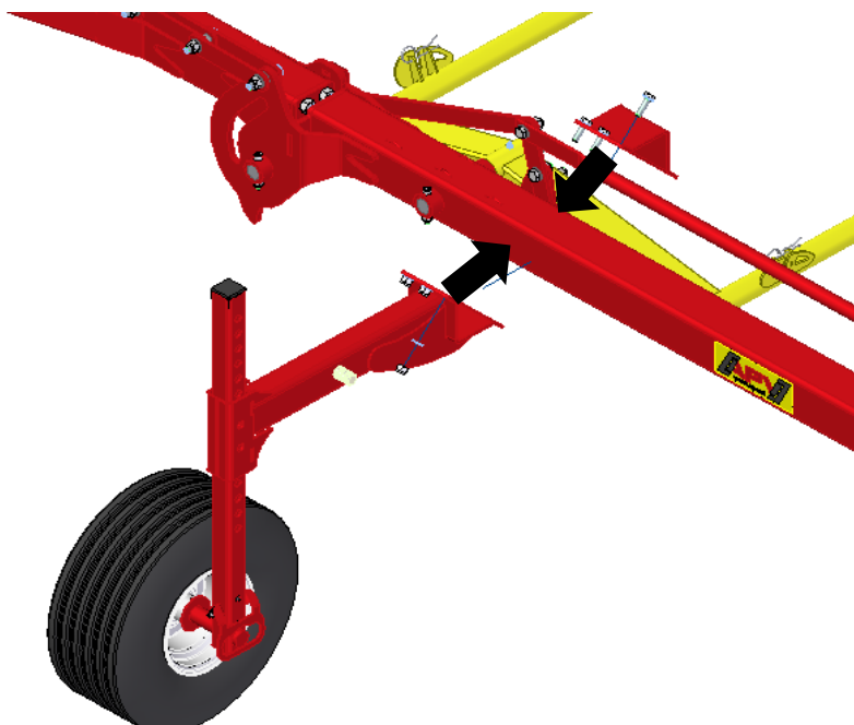
Figure 28: Feeler wheel installation for the AS 1200
