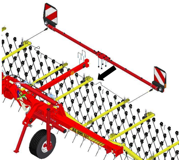
Illustration 11 : montage de l'éclairage AS 600 M1
