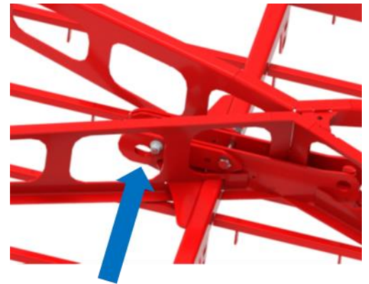
Figure 15: Folding locking plate on the side frame
